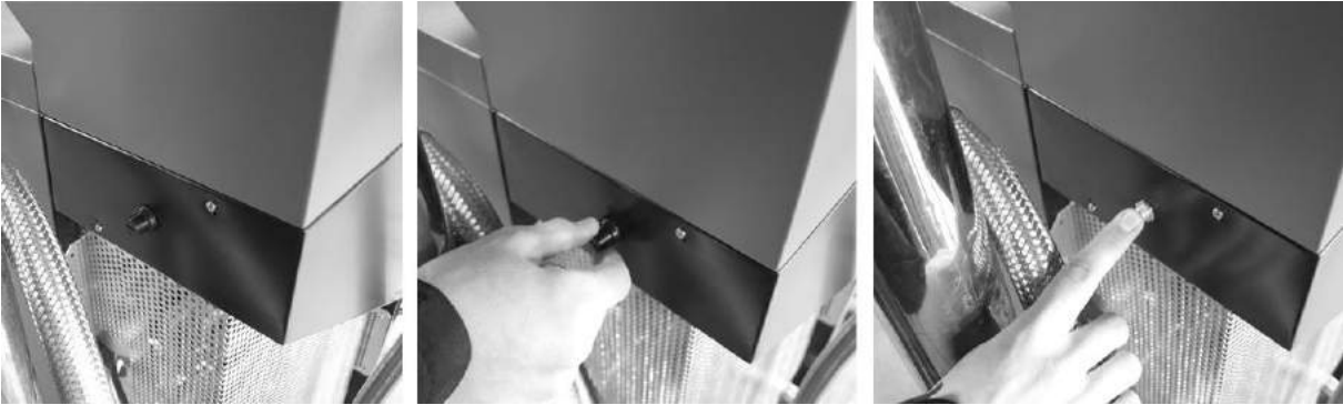
Figure 17: Activating thermal safety
